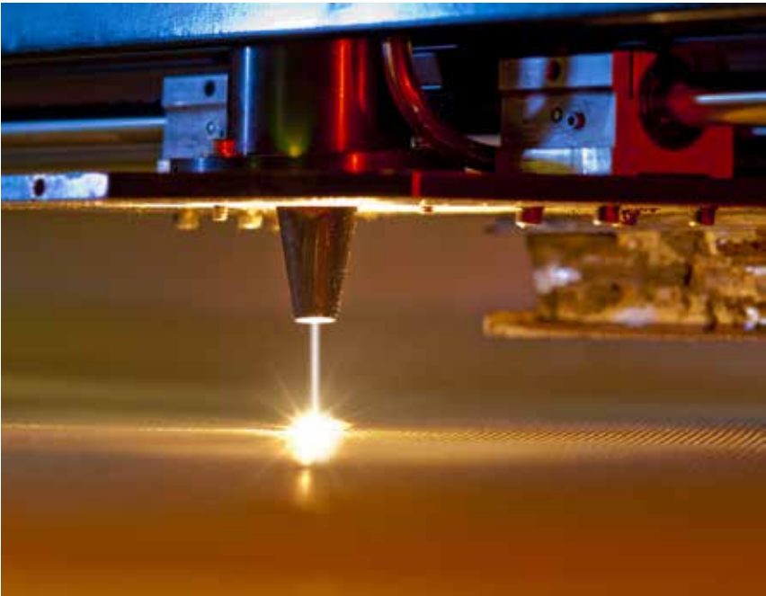
In industry, the power of a laser is used to cut through heavy sheet metal.
